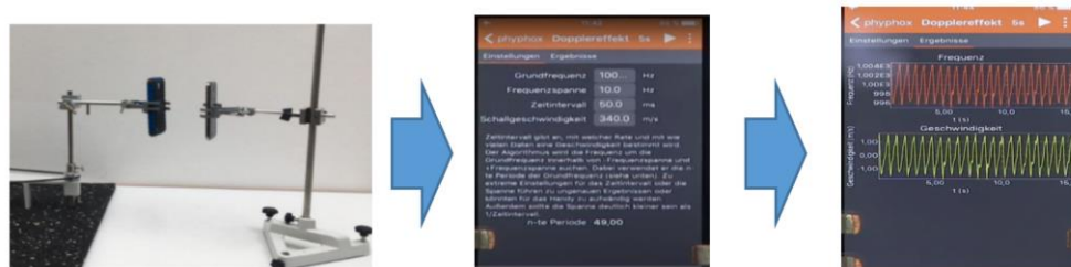
Figure 3 Scheme of basic physics practicum doppler effect basic physics practicum based on virtual android observatory
