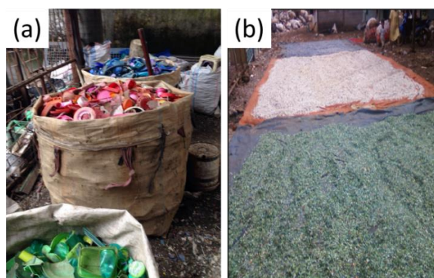
Figure 1. Plastic waste before (a) and after shredding (b) (Courtesy of CV Peka, Jl. Sapan Raya 1A, Bojongsoang, Bandung).
