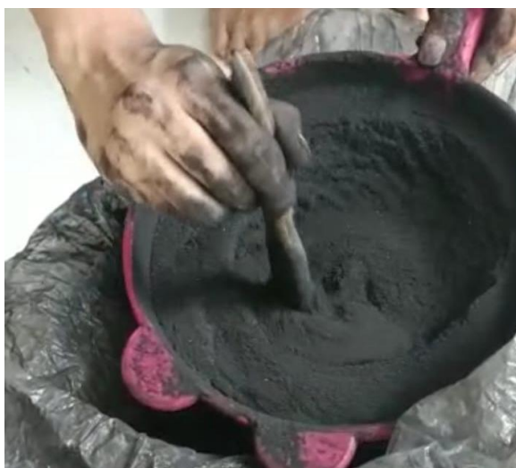
Figure 6. Durian peel charcoal powder sieving process.
