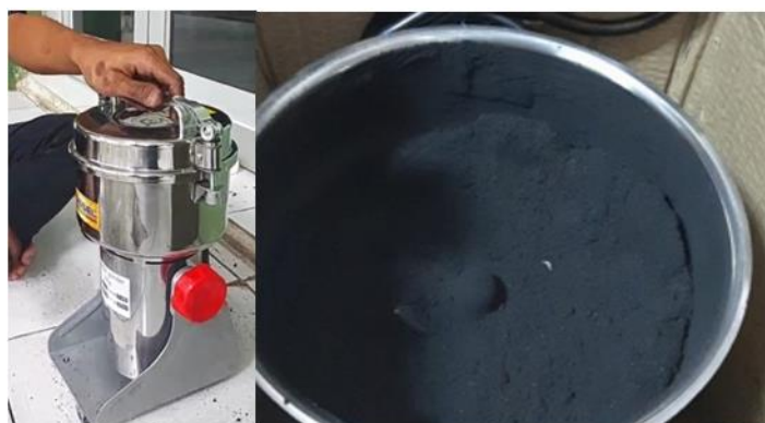
Figure 5. Process of smoothing durian skin charcoal using a powder grinder.
