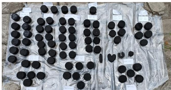
Figure 11. Briquette drying process.
