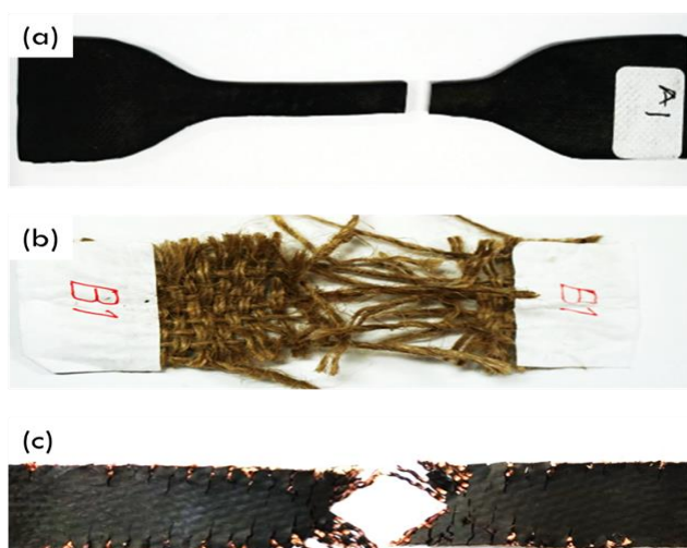
Figure 2. Specimen after tensile tests for (a) base rubber material (b) reinforcement material and (c) composite material.
