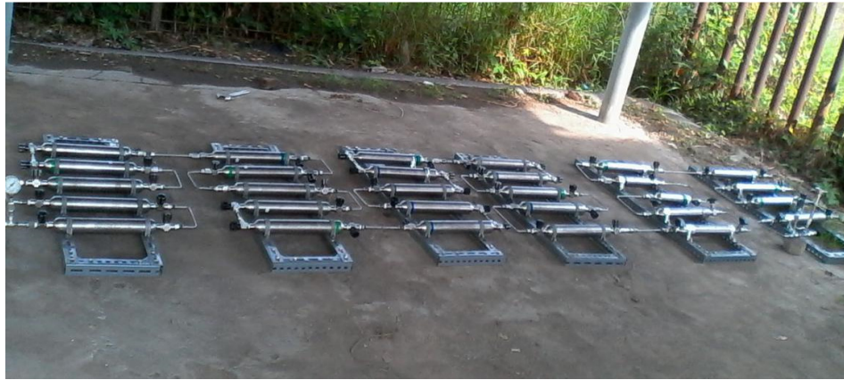
Figure 1. Arrangement of gas cylinders for preparation of PT samples.
