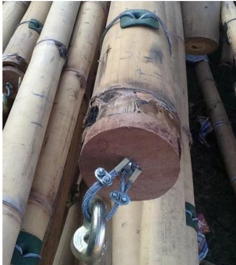
Figure 7. Bamboo radial compression connection (Widyowijatnoko, 2016)
