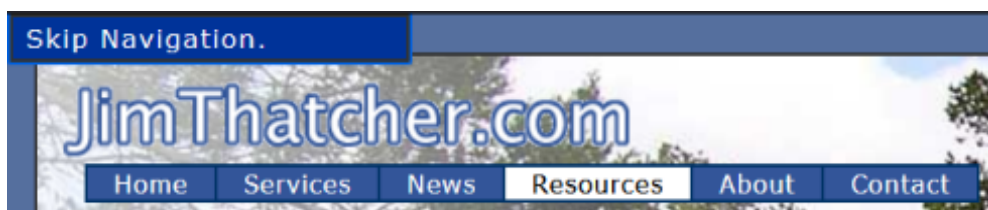
Figure 7. Example of a skip to content element to meet the bypass block criteria
