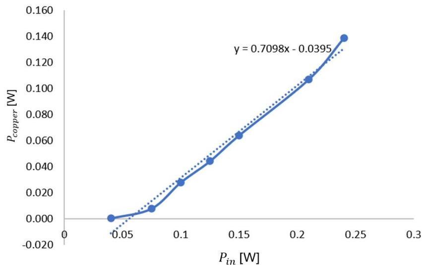
**Figure 3:** Copper Loss Coefficient Evaluation
