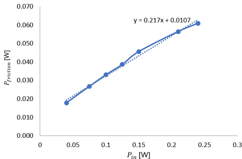
**Figure 2:** Friction Loss Coefficient Evaluation
