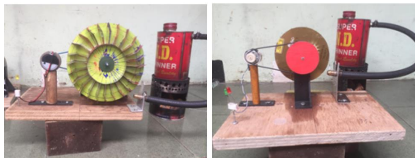
Figure 5. The original design of steam power plant powered by wood sawdust waste.
