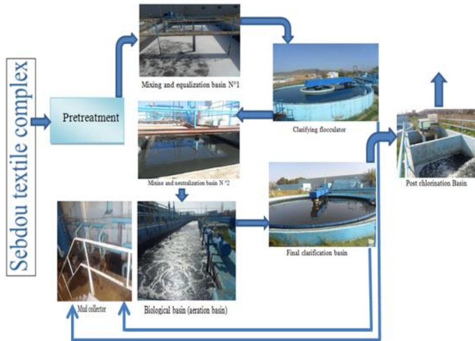
Figure 1. Schematic diagram of the physicochemical treatment process in the station of the textile industrial unit.
