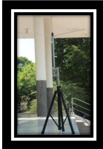
Figure 8. Design and Dimensions of the 5/8 \lambda vertical antenna
