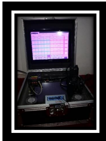
Figure 7d. Portable VSCS communication system
