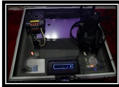
Figure 7c. VSCS communication device on bottom box with acrylic cover
