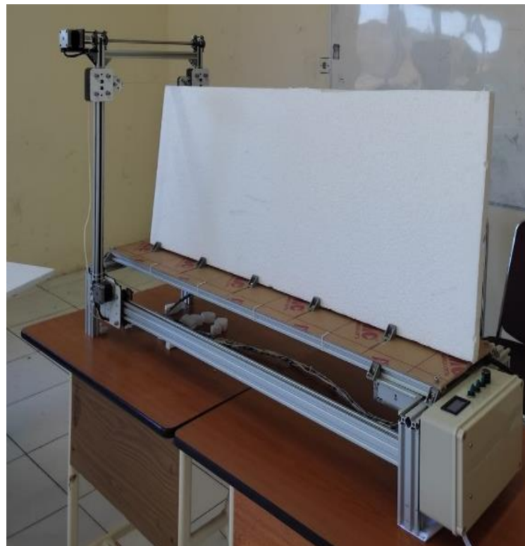
Fig. 1 CNC2 Axis Based Styrofoam Cutting Machine Using Hot Wire.
