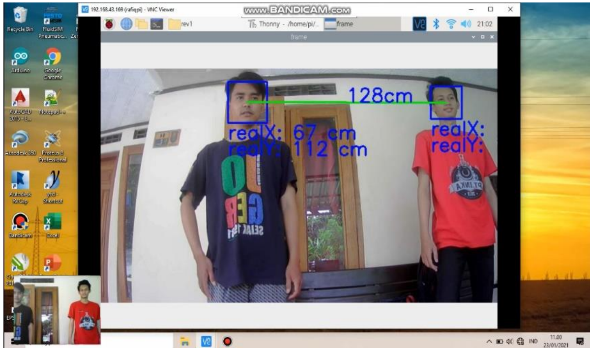
Figure 10. Testing Of Face Distance Exceeding 100 cm.
