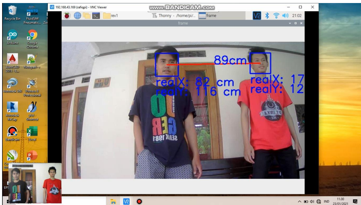
Figure 9. Display of Face Distance Identification Less Than 100 cm.
