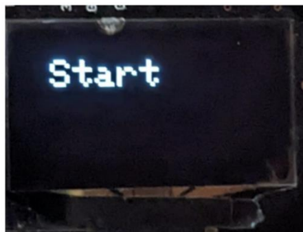
Figure 3. When ESP32 is switched "ON", showing the "Start" word in 1-s intervals before using.
