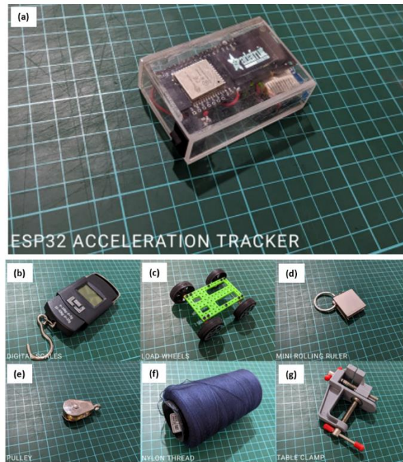
Figure 1. (a) ESP32, "wrapped" by acrylic to attach it by ease in load wheels, (b) digital scales, (c) load wheels, (d) rolling ruler, (e) pulley, (f) nylon thread, and (g) Table Clamp
