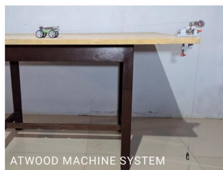
Figure 2. Atwood machine system.
