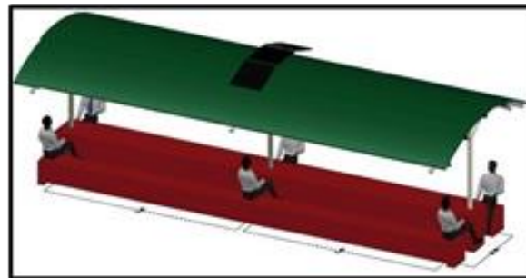
Figure 3. Proposed AutoCAD design of the solar-powered charging station that shows the social distancing between the users.
