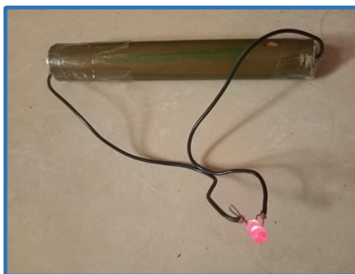
Figure 2. Application of bio battery with fruit electrolyte to LED light.
